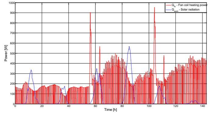
Figure 3 – Fan coil heating power and solar radiation transmitted through the window in the zone.
