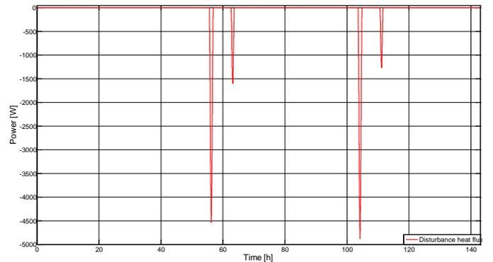
Figure 4 – Disturbance heat flux due to window opening.
