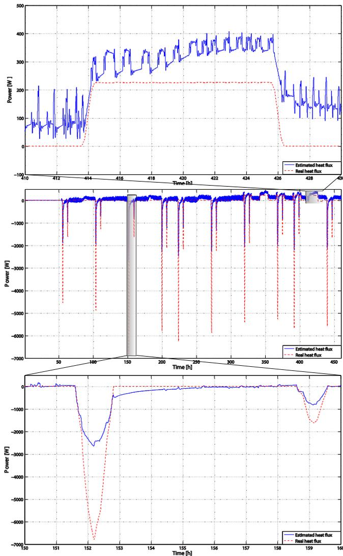
Figure 6 – Estimated and real disturbance heat flux.
