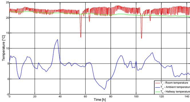
Figure 2 – Zone temperature, ambient temperature and hallway temperature.
